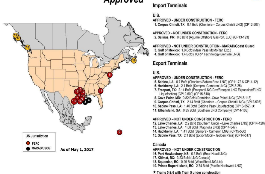
Figure 4. North American LNG Import/Export Terminals Approved. Source: FERC.
